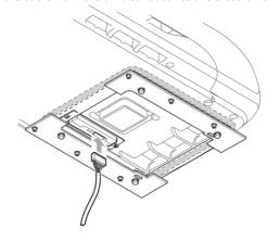
Screw the air distributor (arrow pointing in the vehicle's direction of travel) to the brackets with 6 screws M6 x 12 mm.
