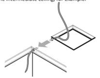
Lift the unit onto the roof, holding it in a horizontal position, and insert it into the cut-out. The arrow points in the vehicle's direction of travel.
