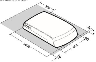
The clearance around the **air distributor** must ensure that air can escape unrestricted. There must be a clearance of at least 40 mm to the side. The swivel range of flaps and doors must be taken into account.
